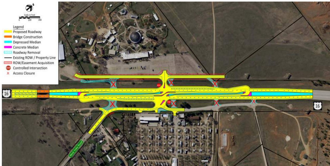
Figure 7: Build Option 1.2a, RCI at Central Driveway
