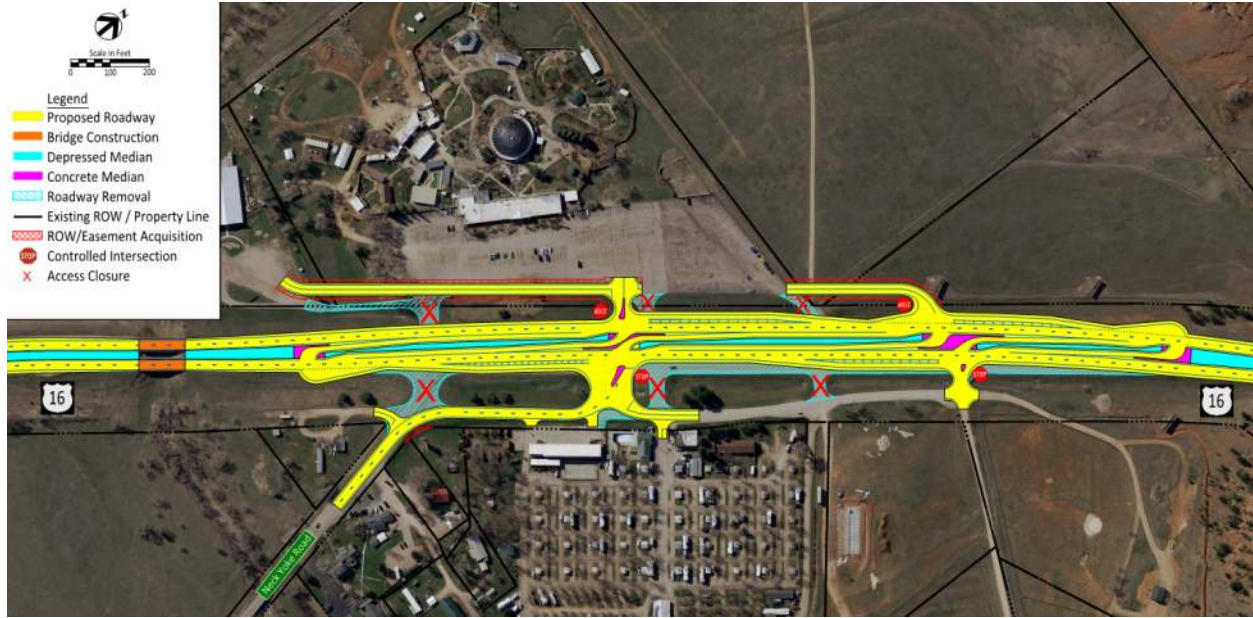
Figure 10: Build Option 1.3b, RCI at Central Driveway with US16 Realignment plus Northern \frac{3}{4} Access
